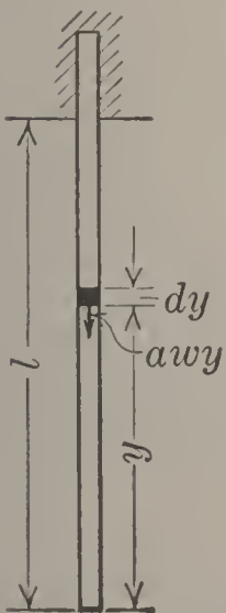
FIG. 17.—Bar stretched by its own weight.
